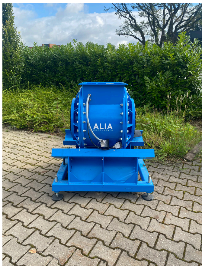
Figure 1. New accelerometer-based slurry density meter.
